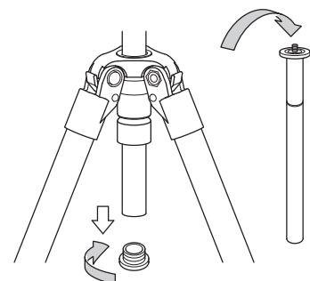
Remove the center column base stopper and pull out the center column.
