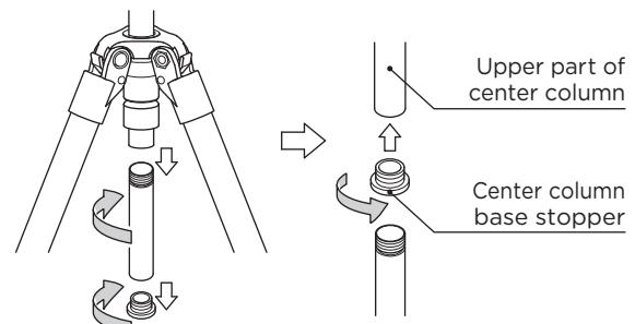
Rotate the lower part of the center column and the base stopper counterclockwise. Attach the base stopper to the bottom of the upper center column to prevent it from slipping out of the tripod.
