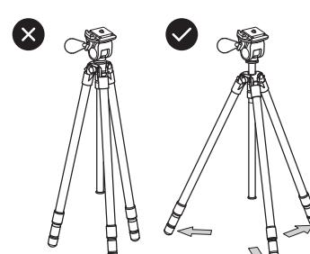
Make sure all levers, knobs and handle are securely tightened before attaching your camera.
