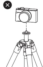
Do not attach a camera directly to the pan head attachment screw as it may damage both the camera and the attachment screw.
