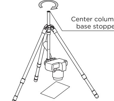
Insert the center column from the bottom of the tripod base and tighten the column lock. Make sure to re-attach the center column base stopper in order to prevent it from slipping out accidentally.
