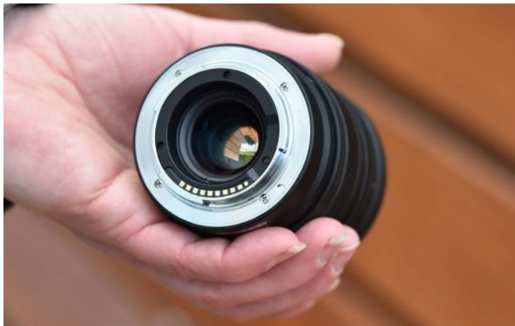
Electrical contacts relay focal length and aperture data to the camera
