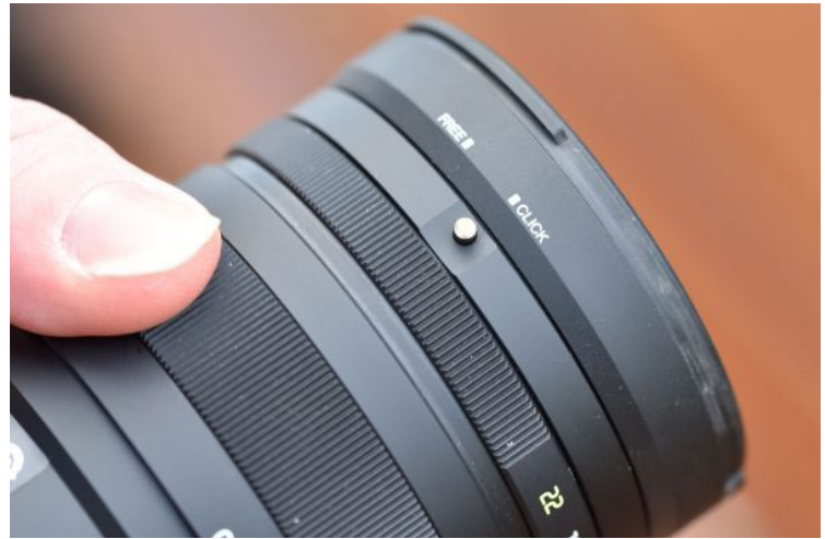
Pressing this small button and turning the collar de-clicks the aperture ring
